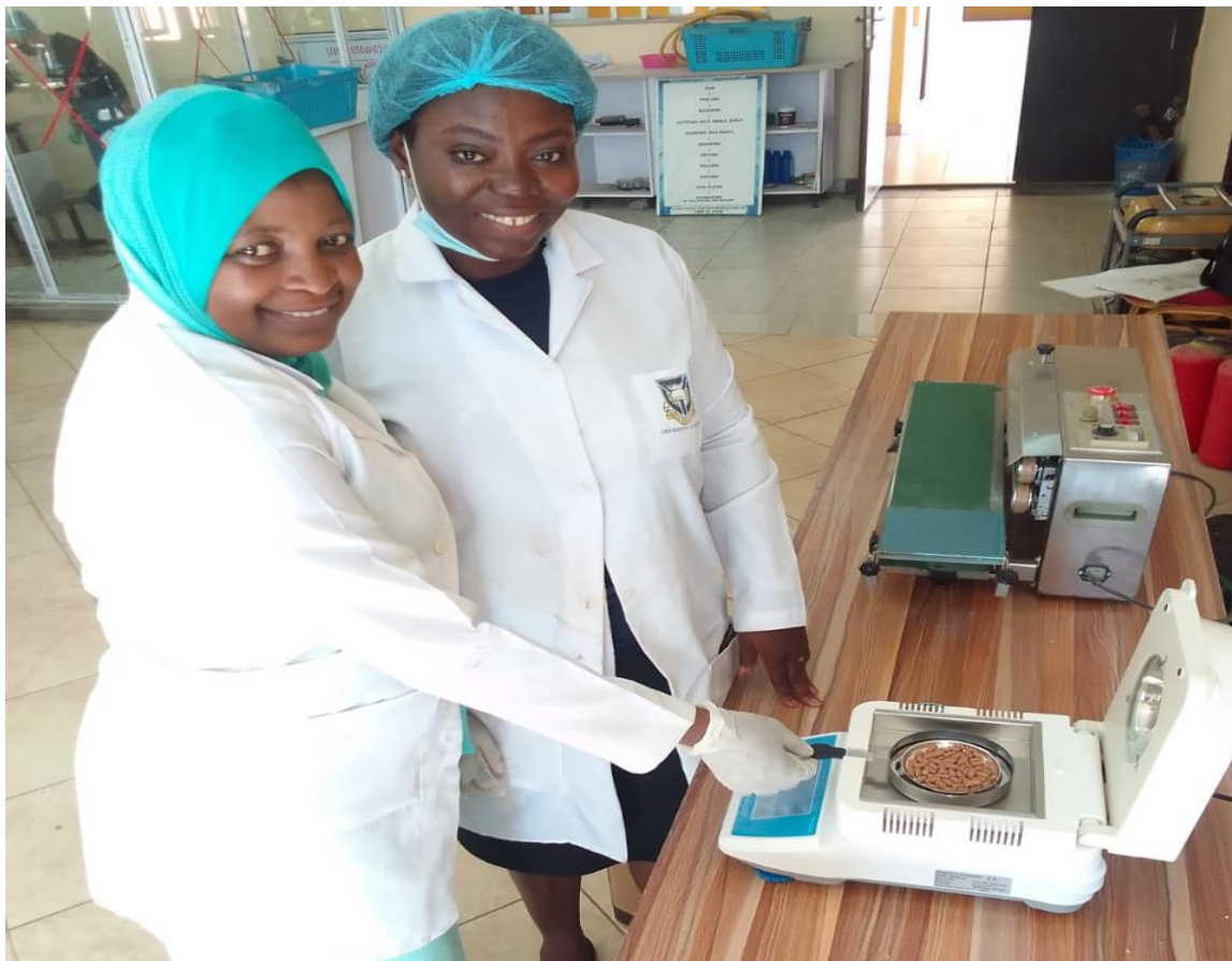
Dr MojisolaOyewole and Dr FolasadeAdeboyejo determining moisture content of extruded products
